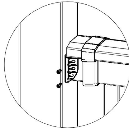
**Step 7 - Secure the top rail.** Position the top rail over the exposed ends of the balusters so that it is positioned on the resting flange of the installed nylon post brackets. Attach the top rail to the nylon post brackets by using the (4) #10 x 1" pan-head screws. Fasten two screws into each side of the nylon post bracket using the top and bottom slots of the nylon post brackets. Snap the alzar bracket covers positioned in Step 6 onto the nylon post brackets.
