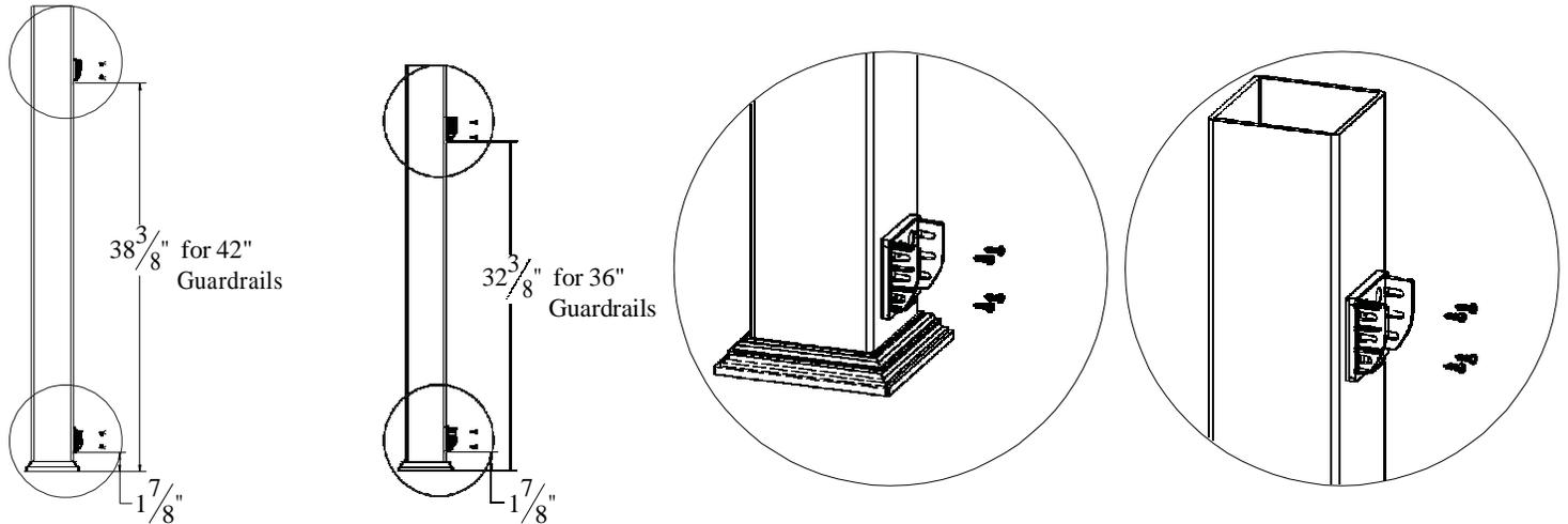
**Step 2 - Secure post mounting brackets.** Attach the nylon post brackets to the sleeved posts by using the (4) #10 x 1-1/2" pan-head screws for the 4" x 4" treated wood post, or the (4) #10 x 1" pan-head screws for the SNL mount. Measure and secure the bottom nylon post bracket 1-7/8" from the installed deck surface. Similarly secure the top nylon post brackets to the installed posts 38-3/8" from the deck surface for a 42" railing heights or 32-3/8" for 36" railing heights.
