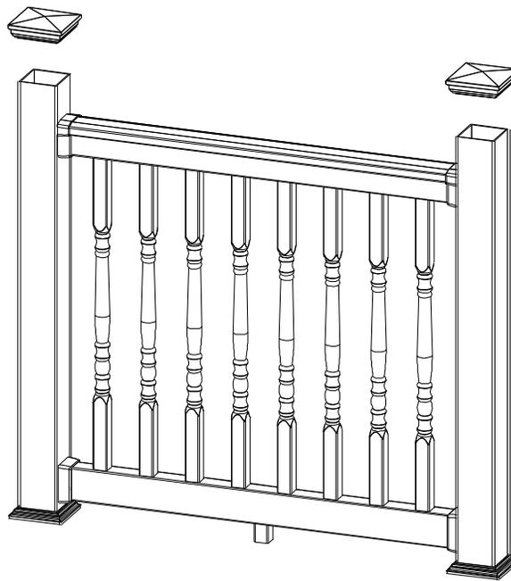
**Step 8 - Finish the section.** Secure the 4" x 4" post caps onto the post tops by applying PVC adhesive to the internal surfaces of the post caps. Set the caps onto the post tops. Wipe off any excess adhesive.
